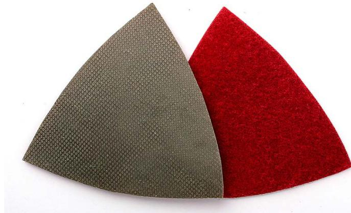
The triangular polishing pads are used for FEIN MultiMaster type oscillation tools for detailed polishing of granite, marble, concrete and other types of stones. They are 3" for each side. The entire set comes with grite 60# 120# 200# 400#. they can be used for wet. the triangle diamond polishing pads are also suitable for Dremel Multi-Max, Rockwell SoniCrafter, as well as Ryobi detail.
