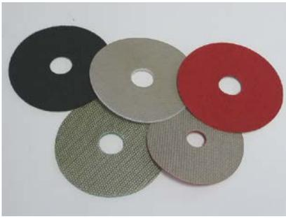
Quick release discs for grinding natural and synthetic stones, glass, ceramics and hard metals. Colour coded for easy grade identification. These quick released (Velcro) flexible diamond discs are for hand and fixed machine polishing. They should be used wet. All sizes and grades available. All other backings and fixings available including M14, snail lock, self adhesive, plastazote and magnetic. Quick release
