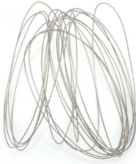
The Diamond Coated Wire Loop is a cutting tool used for cutting graphite in various shapes. Graphite is a versatile material used as electrodes, targets, and other applications. With the use of diamond loop wire, cutting graphite in any shape is possible. The cutting thickness can range from 100-200mm, and the cutting speed is high, reaching 50-60m/s. The feed speed can also reach up to 80mm/min, and the cutting process is dry.
