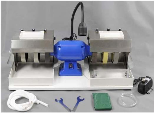
This Cabbings Grinder Machine with 1" stainless steel shafts and ball bearings, 7 pcs Aluminums Spacers and Flanges and locknut. It also has a 3/4HP Thermal protected ball bearing motor, the Hood process by 304 stainless steel. We also can supply a adjustable drip water system with 8 shut off valves for each wheel. The shaft is tapped for a 1/4-20 spin-on polish head at right ends and tapped for a 1/2" Aluminum lap or Diamond
