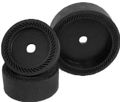
Angled expansion slots through the heavy rubber rim allow the drum to expand when rotated; thereby locking the belt in place. Belts can be quickly changed by stopping the machine, slipping of the old one and sliding on the new. In use, the resilient drum surface flexes to the gemstones contour to quickly remove grinding flats. The convex shaped drum provides the cutting action necessary to remove scratches. Sold without belt.
